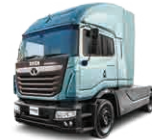
Prima H.55S Industry-first H2 ICE truck for eco-friendly goods transportation
