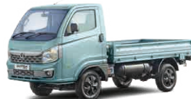
Intra Bi-Fuel India's first bi-fuel pickup offering the dual benefits of CNG and petrol
